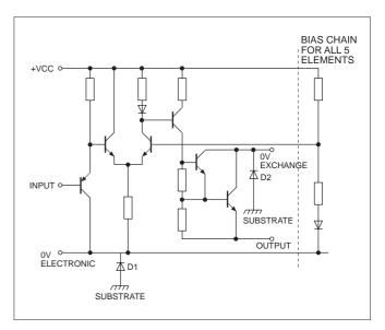
Figure 2: Circuit diagram of one element
