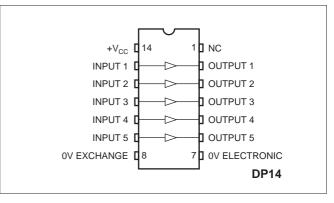
Figure 1: Pin connections (viewed from underside)
